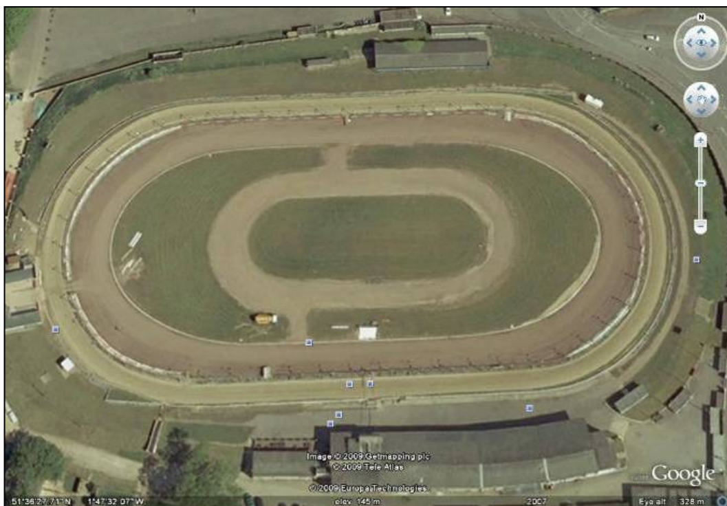
Typical multi-purpose speedway track (Swindon, U.K.), showing junior track inside senior track, which itself is inside a greyhound track.
